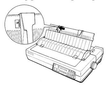
4. Adjust the right edge guide to match the width of your paper. Next, slide a sheet down between the edge guides until it meets resistance.
